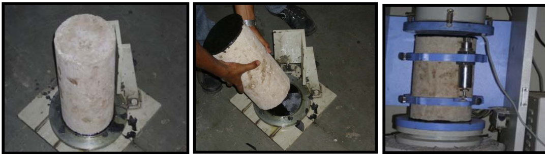
Figure 4: Cylindrical Specimen being tested in compression testing machine after being capped using artite powder
