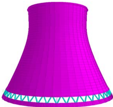
Fig. 11 Finite Element Model of cooling tower
