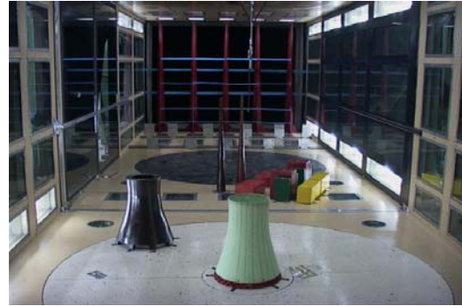
Fig.2 Picture of instrumented NDCT along with other nearby plant structures for interference study in the wind tunnel (typical orientation).
