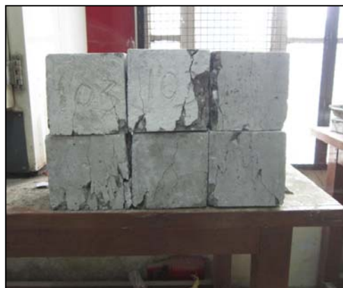
Fig.3: Typical Mode of Failure for Cubical Specimens.
